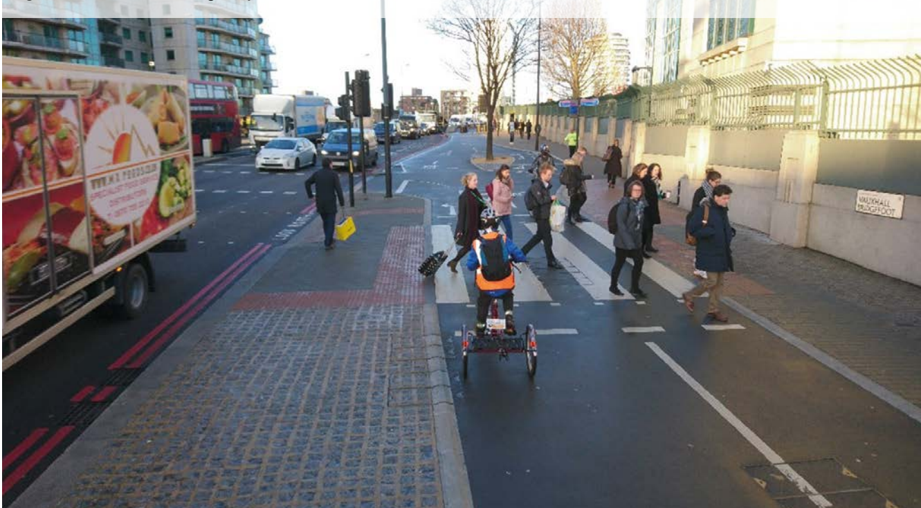
Figure 6.12: Zebra crossing of cycle track, London
