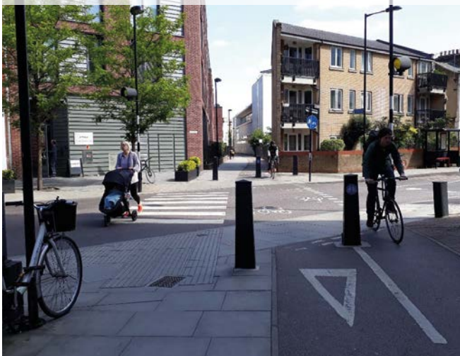
Figure 10.7: Parallel crossing, Hackney
