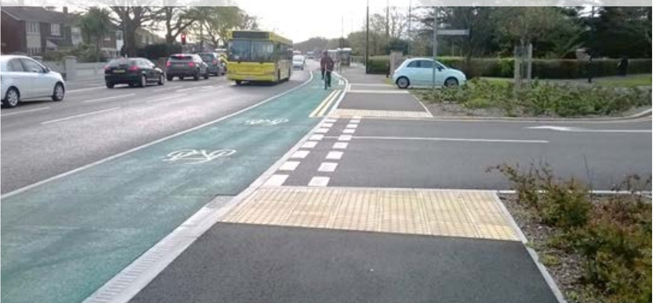
Figure 10.17: No setback crossing with design priority,– Bournemouth
